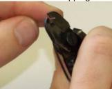
2.2 After removing approximately 20mm of matrix material, it is now possible to separate the fibres ready for the next stage.
