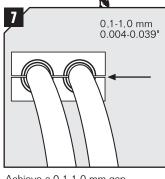
Achieve a 0.1-1.0 mm gap between the two halves when held against the cable.
