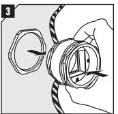
Insert the gland in the hole. Fasten it Pull all the cables through. with the lock nut.
