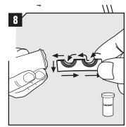
Lubricate all modules for the frame thoroughly with Roxtec Lubricant, both the inside and the outside surfaces.
