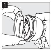
Separate the lock nut from the gland housing.
