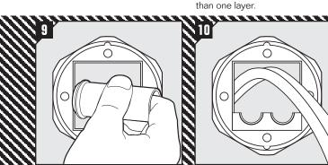
Lubricate the compression rubber. Start b Especially in the corners. the bot
