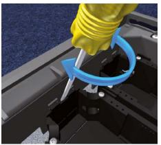
**9** | Releasing device cup Push mounting lever or screwdriver between frame and device cup. Release latches separately sideways and take out device cup.
