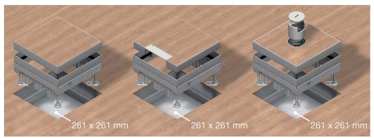
Quadrangular cartridge unit with hem, made of stainless steel, with the outside measurements of 261 x 261mm as a dummy cartridge unit, cable outlet cartridge unit and tube cartridge unit for the installation into screed and hollow floors. For 12/22/32/42 mm parquet and stone covers and linoleum in combination with rigid foam lid insert. Can be levelled from 65 to 315 mm.
