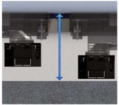
**17 | Maximum installation height** Maximum installation height: 109 mm when using a 50 mm lock-in lead, respectively 134 mm when using a 80 mm lock-in lead.
