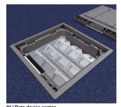
**21 | Data device carrier** Up to nine data modules can be insatlled in the data device carrier using boards in the installation unit. Minimum installation height: 96 mm when using a 50 mm lock-in lead, respectively 116 mm when using an 80 mm lock-in lead set. Use the lock-in lead considering the bending radius.
