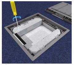
**20 | Device insert** Place device insert into the installation unit from the top and tighten to the frame using four threaded screws. Minimum installation depth: 63 mm. Suitable for maximum two double sockets and up to six data modules. Install installation technology using boards.
