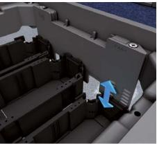
**9** | Lock-in leads Depending on the installation situation, lock-in leads of heights either 50 mm and 80 mm can be chosen. Device cups can be gradually lowered by up to 30 mm.
