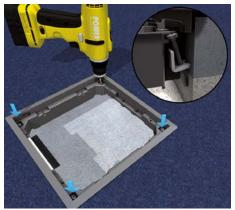
**4** | Fastening the installation frame Insert frame into installation opening from the top and tighten the pre-assembled claws with a crosshead screw. Check to ensure the frame fits tightly.
