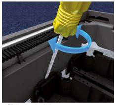
**10 | Releasing the device cup** Insert screwdriver or mounting lever between frame and device cup. Release lugs on the side individually and remove device cup.
