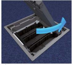
**11** | Inserting the hinged cover Insert hinged cover from the left back side, push firmly backwards on the right and latch in the hinge. The hinged cover can be inserted rotated by 180° and remains open in locking position.
