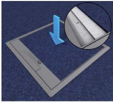
**12 | Floor cover** Cut floor cover to no more than 10 mm from its precise fit and glue onto the steel reinforcement. Optionally, cover inlays in 2 mm or 5 mm thickness are available.
