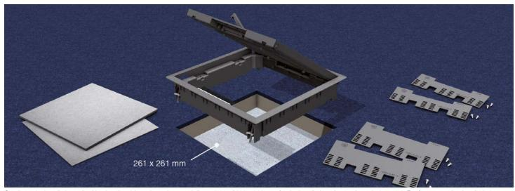
Quadrangular installation unit with a brush cable outlet and external dimensions of 280 x 280 mm for the installation of up to three device cups. For floor cover depths of 10, 8, 5, and 3 mm. Lock-in leads of 50 or 80 mm needed for complementation.
