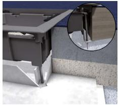
**6 | The use of claws** The claws UDKS 40-80 stretch under the raised floor panel, into the screed or into the cover plate of the floor box.
