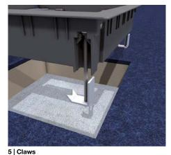
Custom-made applications require the use of claw UDKS 40-80. If that is the case, the pre-assembled claws are removed and replaced. Turn claw body so that the frame can be inserted from the top.
