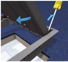
**3 | Hinged cover removal** Open cover completely, pull firmly to the front on the right and release from the hinge using a screwdriver.
