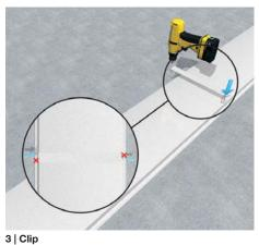
Align duct segments flush and push together. Use one clip per duct joint. Fasten overlapping with two nail plugs. Factor in potential equalization when inserting plugs.
