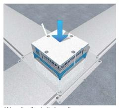
**4** | Inserting the shuttering unit Insert shuttering unit straight from the top into the floor box opening. Floor box and shuttering unit make one mounting unit. Mask all openings in the duct system. Apply insulation flush to duct system and to shuttering unit.
