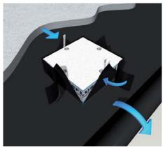
**5** | Screed work / Subsonic noise insulation The shuttering unit must be sprayed with formwork oil. The underfloor system must be insulated against subsonic noise. Mask the shuttering unit with foil. Foil thickness must be < 2 mm. Apply screed neatly to the shuttering unit.
