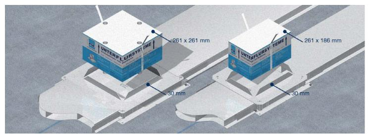
Hollow space floor box for quadrangular installation units 258 x 258 mm or 258 x 184 mm and underfloor ducts of up to 250 or 350 mm width with the heights 28/38/48 mm. Comply with minimum screed covering of 35 mm.
