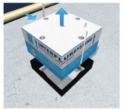
**6** | **Removal of shuttering unit** Remove shuttering unit with the release cord from the hardened screed. Process floor cover to the cleaned installation opening (261 x 261 mm, 261 x 186 mm).
