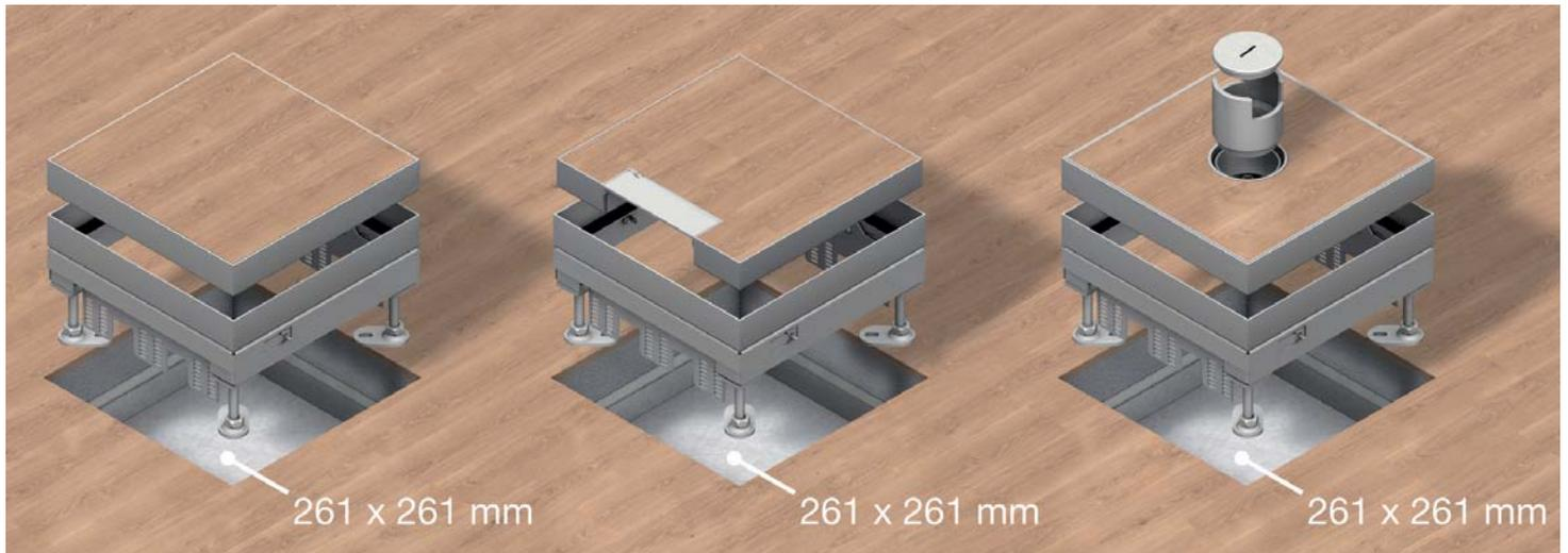
Quadrangular cartridge unit with hem, made of stainless steel, with the outside measurements of 261 x 261 mm as a dummy cartridge unit, cable outlet cartridge unit and tube cartridge unit for the installation into screed and hollow floors. For 12/22/32/42 mm parquet and stone covers and linoleum in combination with rigid foam lid insert. Can be levelled from 65 to 315 mm.
