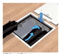
**4 | Rubber seal / Device cup**Glue the rubber seal to the impact-noise interface. Snap the device cup as deep into the lock-in leads as
