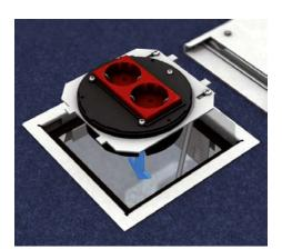
5 | Inserting of device cup Insert plate with the pre-mounted and loaded device cup through the plate slide as deep into the lock-in leads in the frame as possible. A gradual lowering of the plate to max 20 mm possible.
