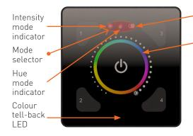
Saturation mode indicator Intensity and saturation horseshoe control / Hue (colour) control circle (depending on selected mode) 193PB
